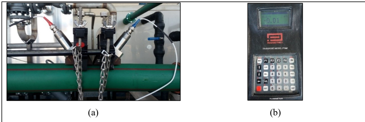
Figure 19 – Photographs of the applied flowmeter sensors (a) and the GE Panametrics PT868 signal acquisition system (b).
